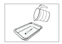
Leave to soak for 10 minutes at 71.6°F ±3.6°F (22°C ±2°C). This procedure reduces the amount of blood, protein and mucous present on the air-polishing handpiece.
