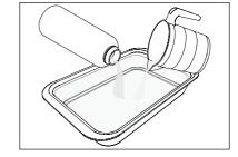
Place the scaler handpiece, front cone, and light guide in the ultrasonic tank immersed in the enzymatic detergent solution at 71.6°F ±3.6°F (22°C ±2°C) and run a cycle for at least 10 minutes.
