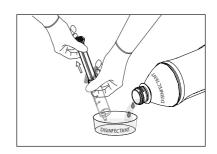
Connect the syringe to the end of the hose previously connected to the male water connection.
