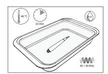
After 10 minutes of immersion in the ultrasonic tank with demineralised water. rinse the internal channels of the airpolishing handpiece by injecting 20 ml of deionised water at ambient temperature 68°F - 77°F (20°C - 25°C) using a syringe with needle, five times in a row.
