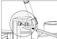
Clean and eventually dry accurately the o-ring seat, by blowing compressed air.
