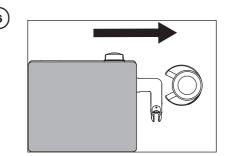
Disconnect the pedal from the device: grab the pedal connector, press the release clip and pull the connector back.
