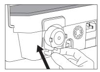
Refit the plastic protection onto the peristaltic pump.
