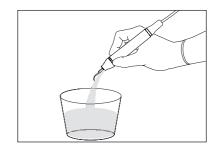
To enter the flushing mode, select "pump/flush" menu on the touch keyboard: all the other selection options present on the display are disabled.
