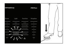
As soon as the peristaltic pump starts working, the entire scale of values in the "irrigation" section lights up, and during the passage of the liquid, the irrigation value switches from 6 to 0.
