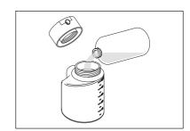
Check that the hose connected to the bottle's cap is correctly installed, then screw the cap back on its bottle.
