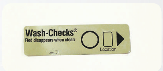
Figure 5. Complete removal of red test soil on Washer-Disinfector Cleaning Monitor after cleaning instruments at Hydrim P3-Heavy Duty Cleaning Cycle.
