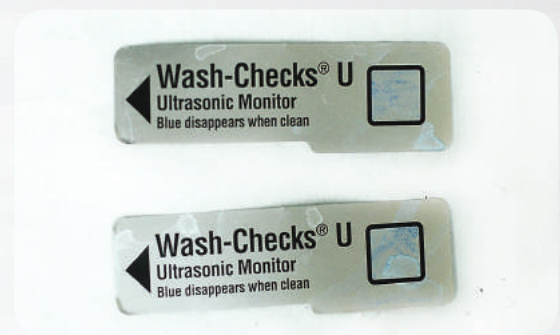
Figure 4. Residual blue test soil on Hu-Friedy Ultrasonic Cleaning Monitors after blood-soaked instruments were exposed for 1 minute in ultrasonic unit.
