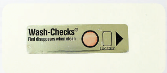
Figure 6. Residual red test soil on Washer-Disinfector Cleaning Monitor after blood-coated instruments were exposed to P1 Rinse-Hold Hydrim cycle.
