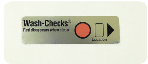
Figure 2. Unused Washer-Disinfector Cleaning Monitoring
